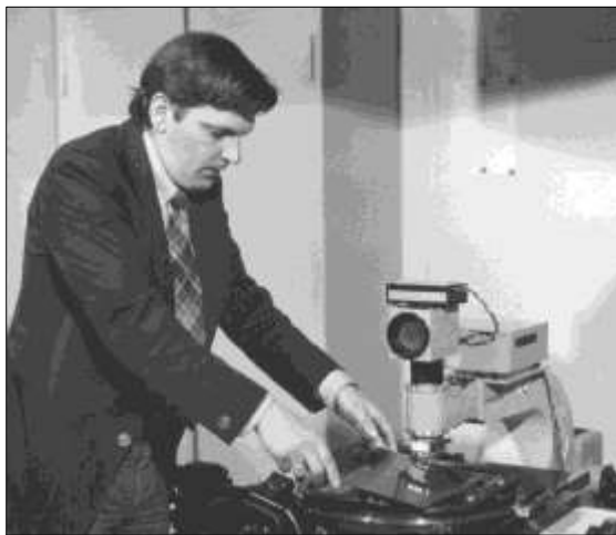
Figure 11: Here I am positioning a 10 × 10-inch photographic plate from the Palomar 48-inch telescope on the plate holder of the Astroscan of Leiden Observatory. The instrument scanned predefined areas with square pixels of 30 microns (corresponding to 2 arcsec on the sky) on a side (From my private archives).
