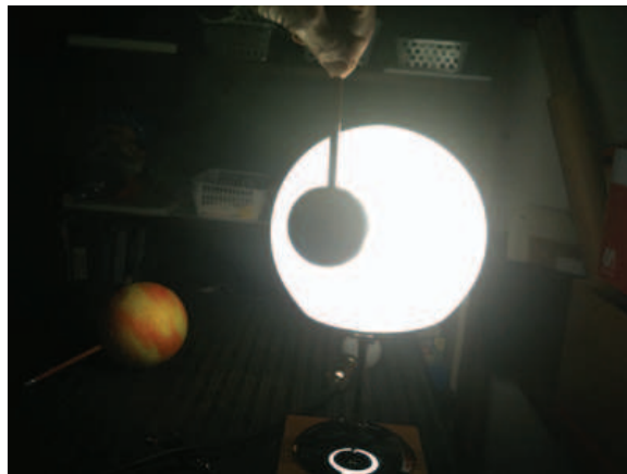
Figure 2. A globe lamp is mounted on a wooden block. Demonstrators pass styrofoam “planets,” held at the ends of pencils, in front of the “star” to simulate a transit.
