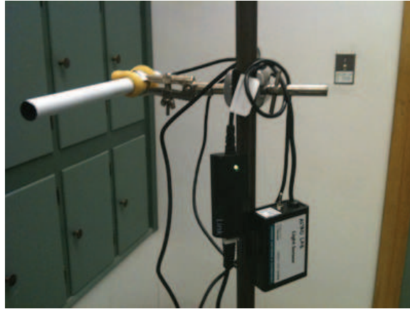
Figure 1. The Vernier light sensor is inside a tube of paper to block scattered light. The sensor connects through a Go!Link interface to the computer USB port.
