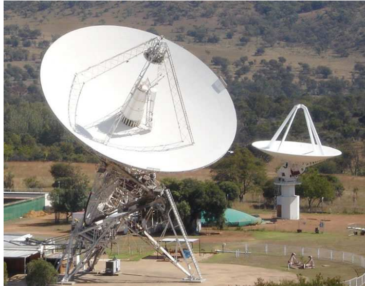
Figure 2. HartRAO with the 26m dish and the 15m eXperimental Development Model (XDM) test-bed prototype for KAT (credit: Mike Gaylard)
