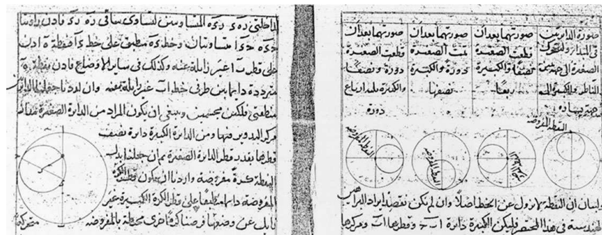
Figure 9. Statement of four different stages of the Tūsi Couple (right), and the proof of the general condition (left).
