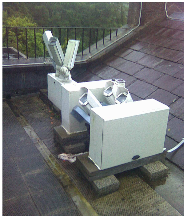
Figure 6 – Meteor video cameras at Armagh Observatory (three cameras in back). In front is the three-camera system of the Polar Bear Telescope.
