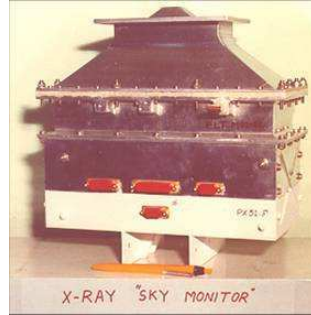
Figure 8. X-ray sky monitor launched on second Indian satellite BHASKARA.
