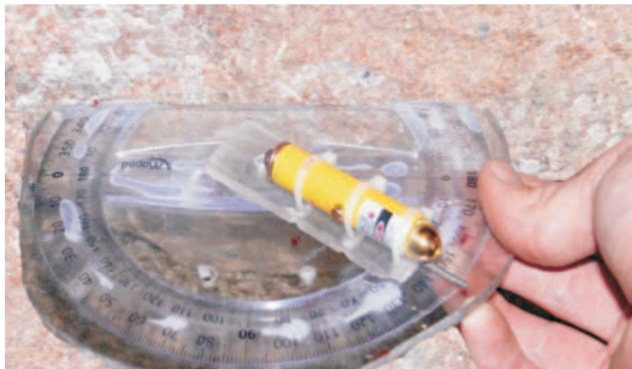
Figure A1. Orientation device used to accurately orientate samples underground. The flat end of the device is placed along the strike of the rock and the laser pointer is then pointed towards the survey peg, where the bearing is read off.
