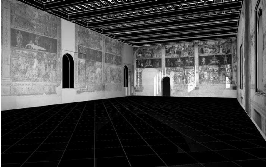
Figure 4. 3D modeling: the sun path in the area dedicated to Borso on the day October 1 st of the XV th century. In that date the figure of the duke is illuminated more times by a strip of light. Such scenographic effects could be opportunely highlighted just by choosing which of the internal shutters should open.
