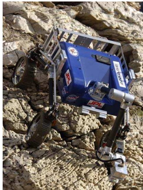
Fig. 3: The Cliffbot Rover moving down the outcrop in the Ebbadalen Formation. The robotic arm with the scoop and the microscopic imager can be seen at the bottom of the image.
