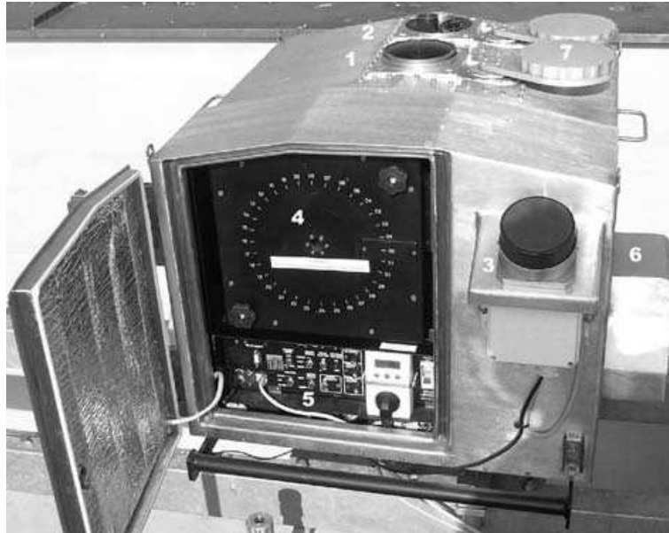
Figure 1. The Autonomous Fireball Observatory. 1–fish-eye lens; 2–battery of sensors (for cloudiness, sky brightness and sound); 3–precipitation detector; 4–rotating cartridge with films; 5–control panel; 6–fans for cooling; 7–covers.
