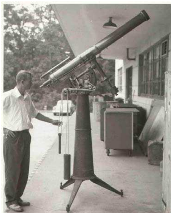
Figure 2. A 5-inch Alvan Clark refractor, one of eight manufactured for the American transit-of-Venus expeditions. Pictured here with Alfred Mikesell at the U. S. Naval Observatory in 1965.
