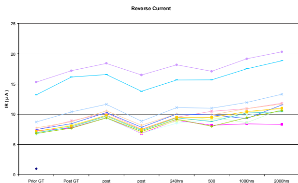
Figure 6 Reverse Current for the Schottky diode 1N5819
