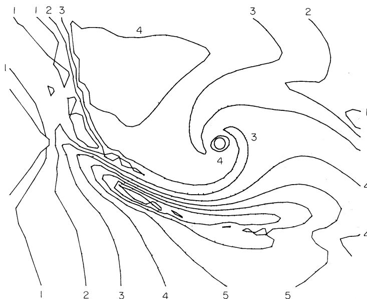
Figure 5. Mach number contours at t = 35 .
