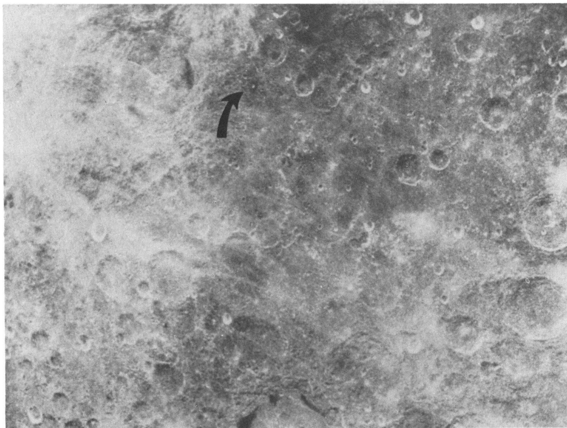
Fig. 4. Light plains region near the crater Balmer (20°S, 70°E) displaying dark halo craters (arrow) indicating the presence of a buried mafic unit. This region also has a high Th content. (AS 17-152-23332).
