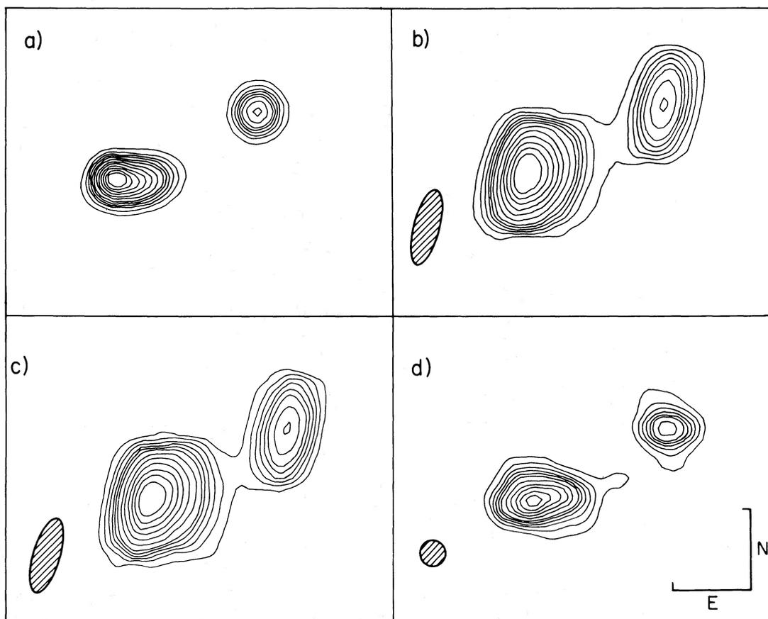
FIG. 7.—Test 5 [( $u, v$ ) coverage, Fig. 2b]. (a) True distribution. (b) CLEAN solution. (c) Hybrid map using closure phase. (d) same as (c) except for the shape of the clean beam. (Contours as in Fig. 3a.)
