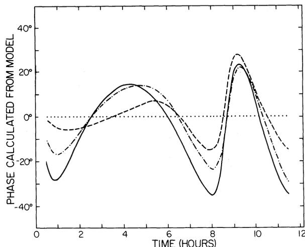
FIG. 3*b*.—A comparison of the phase calculated from the model with the true visibility phase (solid line) on the NRAO-Fort Davis baseline. Dots, first iteration; dashes, 2d iteration; dash-dot curve, 4th iteration. The 12th iteration is indistinguishable from the solid line.
