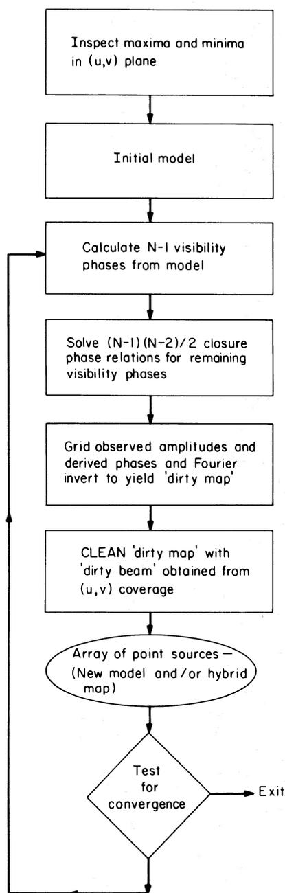
FIG. 1.—Flow diagram of the image reconstruction procedure.
