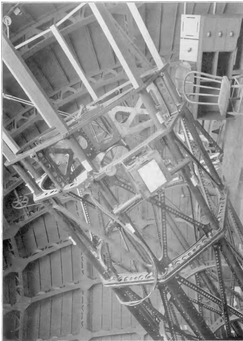
DOUBLE-SLIDE PLATE-CARRIER IN PRINCIPAL FOCUS OF 60-INCH REFLECTOR
