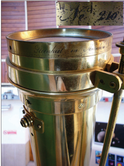
Figure 10: The objective of Tempel's telescope. The engraving on the brass ring holding the objective states: "Steinheil in München N. 216". The production number is on the right side of the ring (a close-up is shown on the top right).
