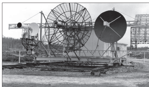
Figure 7: The focal equipment of the first section of the radio telescope. The focal diffraction spot forms on paraboloids which concentrate the radiation on circular horns followed by the high-frequency stages of the receivers (see, also, Figure 8). The intermediate frequency signal is sent to the focal laboratory shown at the back of this photograph. The whole is moveable on N-S rails for focussing. From left to right are devices for 6, 21 and 13cm respectively. The tiltable mirror in visible in the background.
