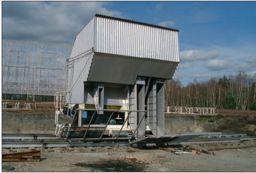
Figure 16: The focal carriage bearing the 21, 18 and 9cm hog horns in the 1980s.
