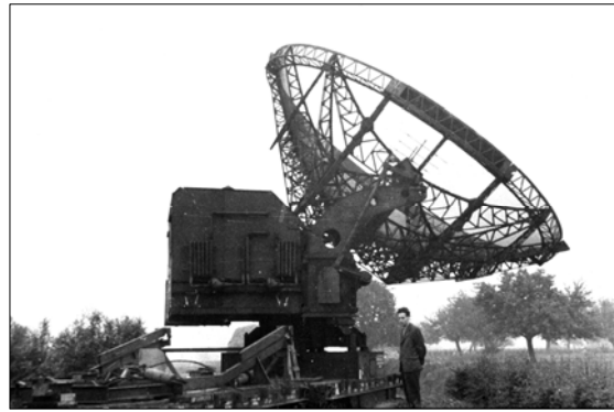
Figure 3: The first of the 7.5m Würzburg antennas mounted on a wagon at Marcoussis and ready for use. Providing an indication of scale is a youthful Jean-Louis Steinberg (courtesy: Observatoire de Paris, Meudon).
