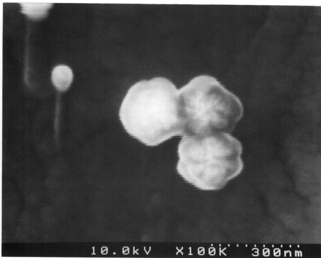
FIG. 6.—SEM images of carbon grains collected after 150 minutes of plasma exposure. The discharge was operated at 5.5 \times 10^{-4} bar argon pressure and 110 W RF power. Note the coagulated grains and the neck formed between them. The beam voltage of 10 keV used in the SEM for this and some other figures altered the surface texture of the grains, smoothing them so that they do not resemble a cauliflower.
